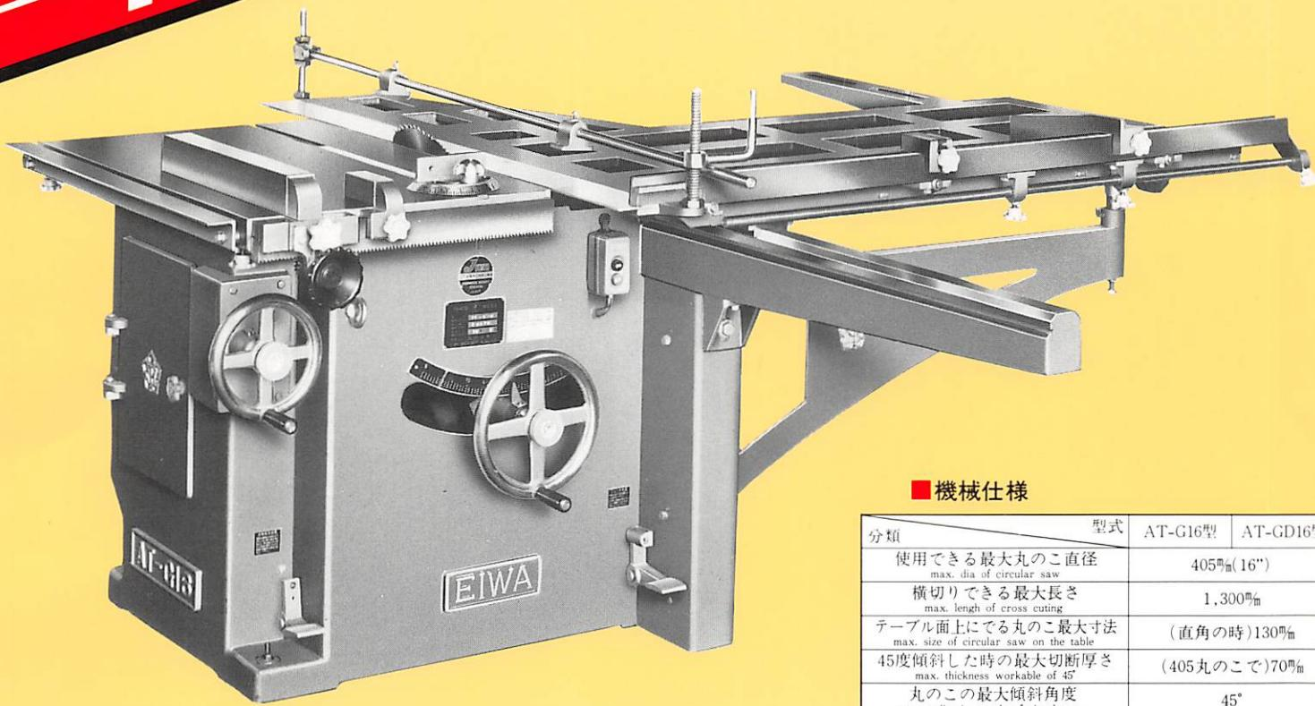
This is a multi-purpose tilting arbor type circular saw on a tilting table base, equipped with sliding table and designed in consideration of safety and workability for the operator.
